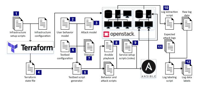
Figure 9: Technical implementation of the model-driven testbed and log data generation approach. Simple arrows indicate imports and filled arrows indicate generation of resources such as scripts, configuration files, or machines.
