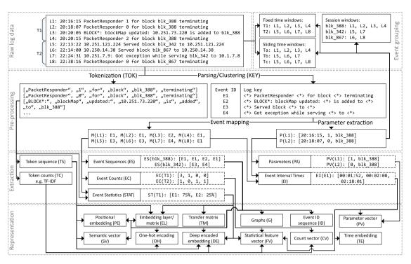
Fig. 3. Different stages of data preparation to transform raw log data into numeric vectors.
